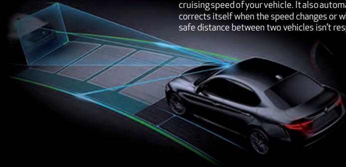
The Active Cruise Control allows you set your the cruising speed of your vehicle. It also automatically corrects itself when the speed changes or when the safe distance between two vehicles isn't respected.
